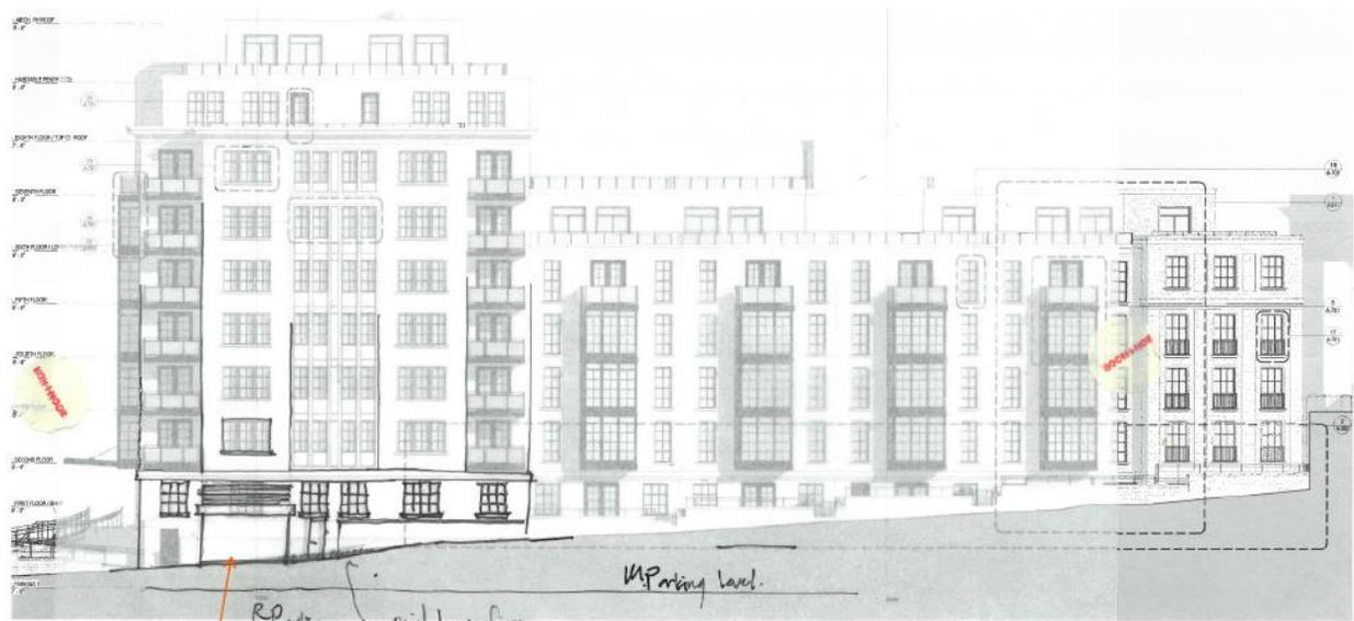
20'-0" wide opening aligns with facade above and improves vehicle/pedestrian sight lines.
